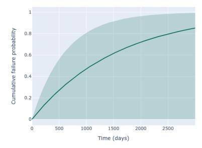
Figure 3. Cumulative failure probability distribution of one WASH on Wheels maintenance activity, based on the data from the follow-up visits, and assuming an exponential distribution. The green area represents the one-sided 95% confidence interval.
